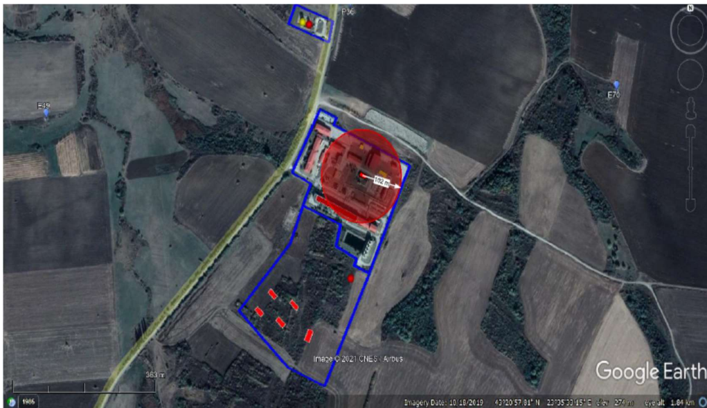
Figure II.3.2-6 Flaring hazard zone in an existing gas drying installation
