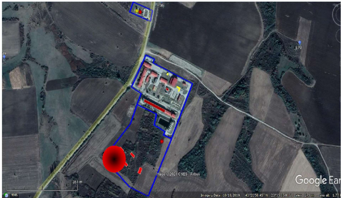
Figure II.3.2-5 Flaring hazard zone in the area of new compressors
