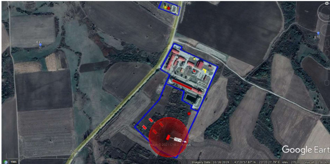
Figure II.3.2-7 Flaring hazard zone in the new gas drying installation
