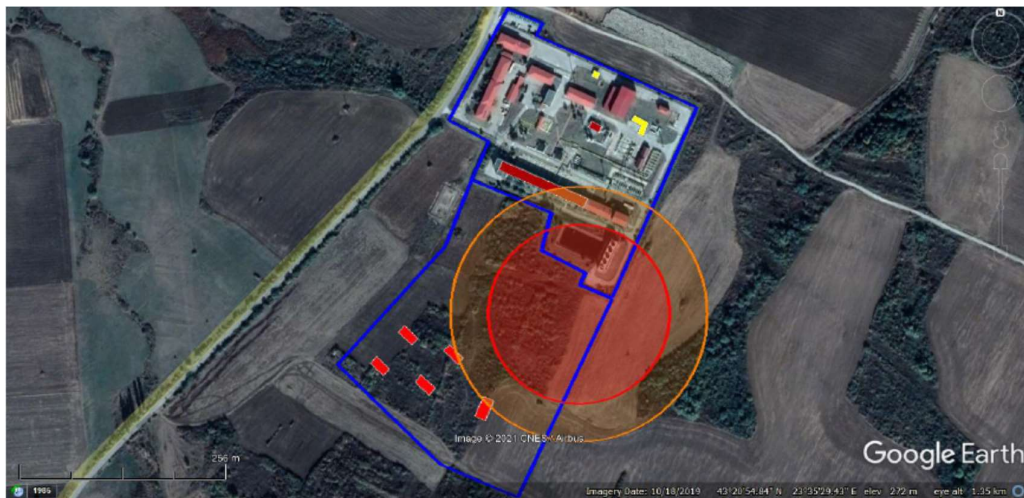
Figure II.3.2-12 Fireball damage zones involving 23.7 t of methanol - production site extension
