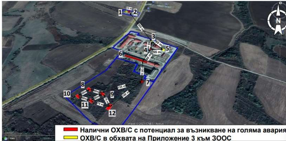
Figure II.13-1 Map of the site of “Bulgartransgaz” EAD with the locations where a major accident may occur and the distances between them
