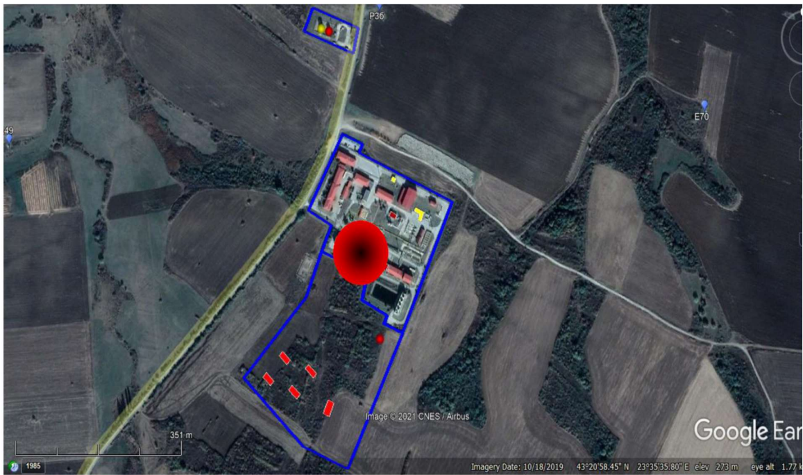
Figure II.3.2-4 Flaring hazard zone in an existing compressor room
