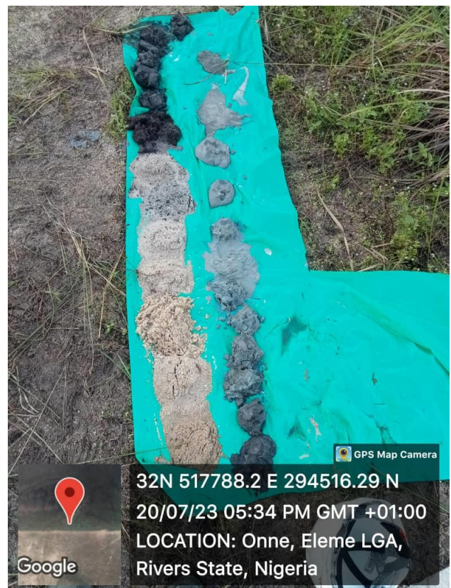
Figure 2.3 soil samples spread across various depths prior to logging
