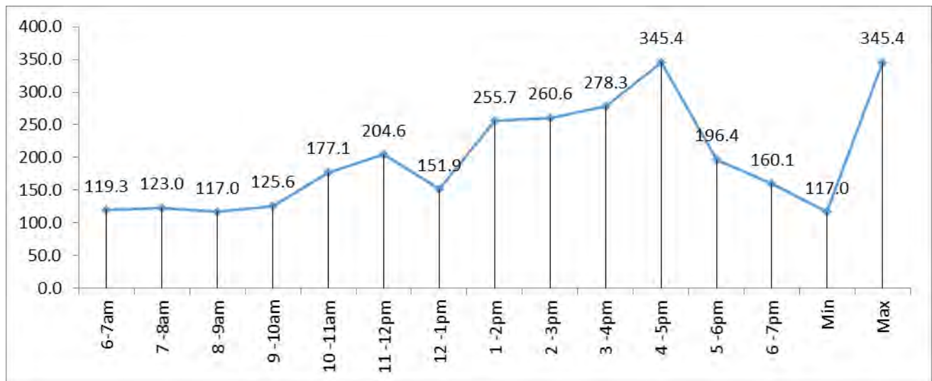
Figure 4.47b: Weekly average hourly traffic volume of vehicles leaving NPA Main Entrance (Out)
