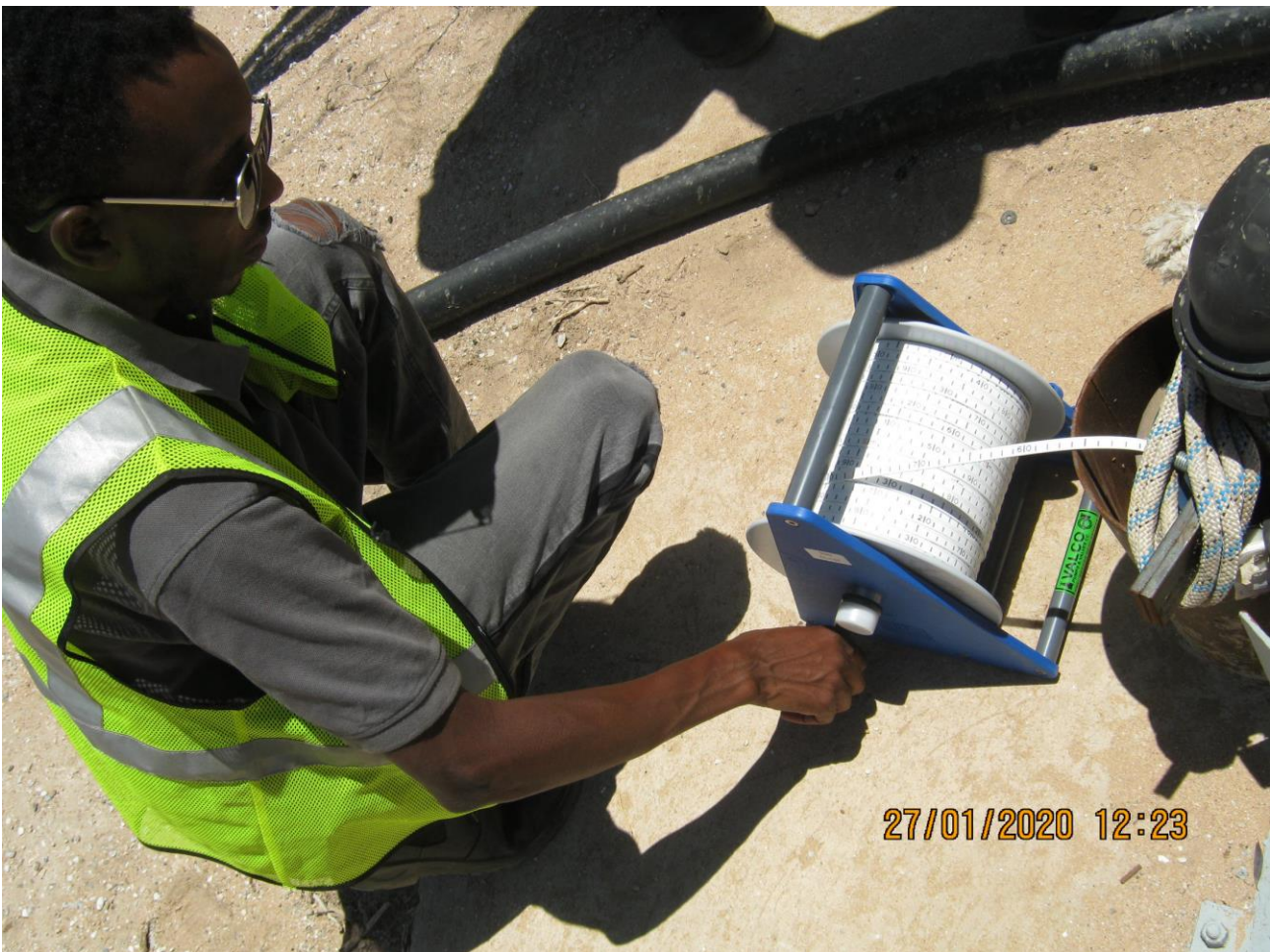
FIGURE 8 – A PHOTOGRAPH SHOWING PERSONNEL FROM ECC MEASURING THE BOREHOLE WATER LEVEL WITH A DIP METER
