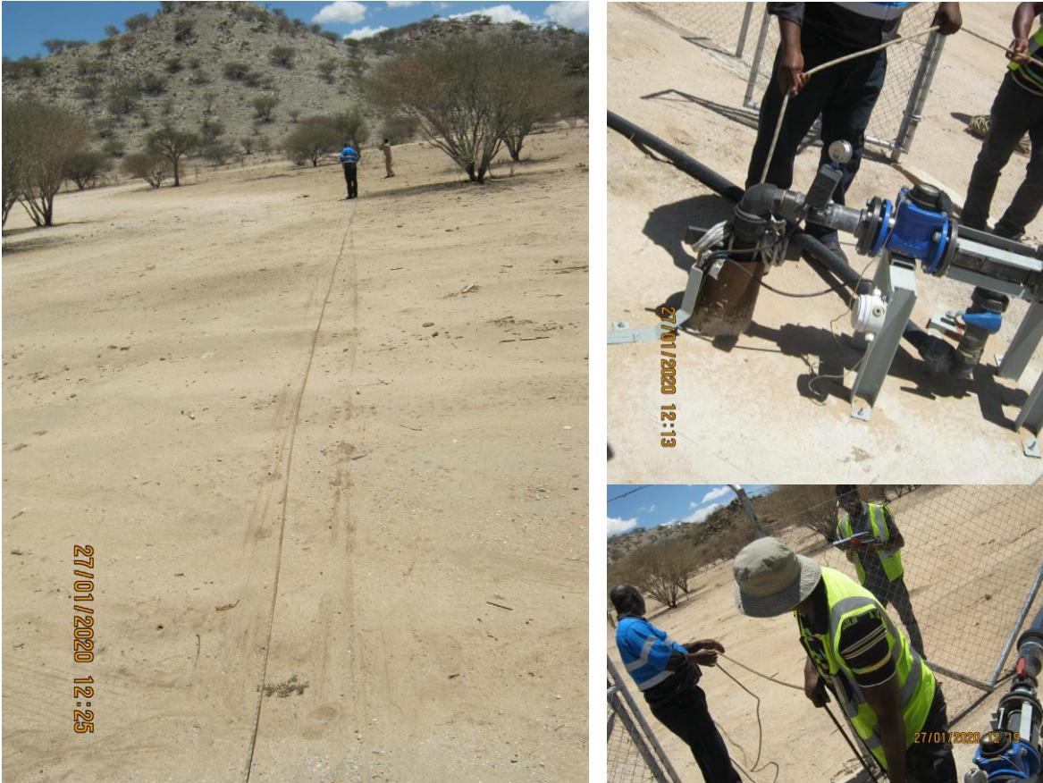
FIGURE 9 – PHOTOGRAPHS SHOWING THE BOREHOLE WATER LEVEL MEASUREMENT BY USING A MAKESHIFT ROPE SYSTEM
