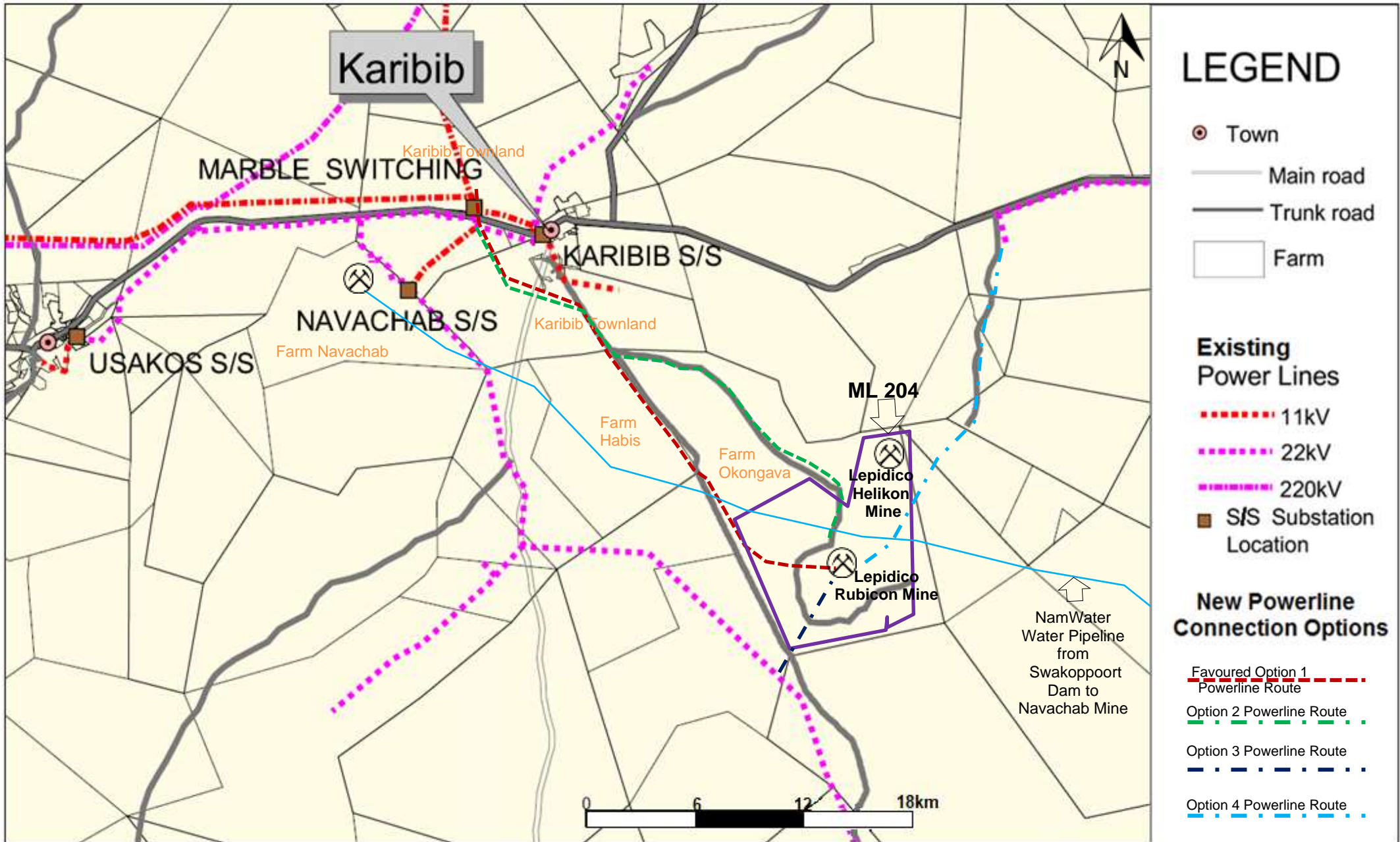
Figure 1.4: All alternative powerline routes that have been considered in bring power supply to the ML 204 (Lepidico Chemicals Namibia (Pty) Ltd Rubicon and Helikon Mining sites) (Source: Lepidico Chemicals Namibia (Pty) Ltd, 2020).
