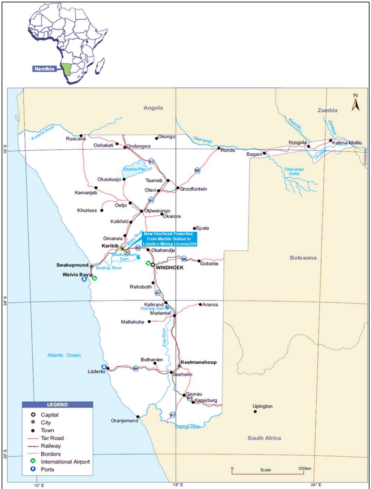
Figure 1.1: Regional location of the proposed 29.977km 66kV overhead powerline from Marble Station to the Mining License (ML) No. 204 of Lepidico Chemicals Namibia (Pty) Ltd.
