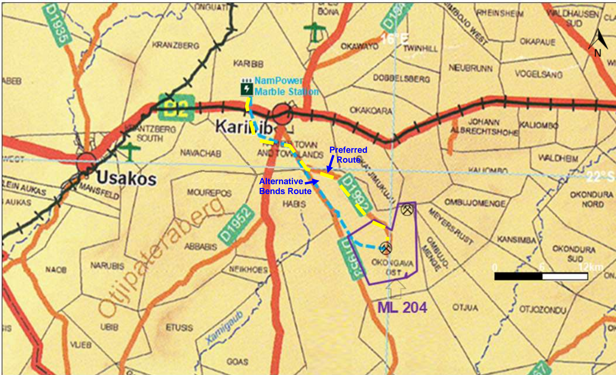
Figure 1.3: Farmlands being cuts across by the proposed 29.977 km 66kV overhead powerline from Marble Station to the Mining License (ML) No. 204 of Lepidico Chemicals Namibia (Pty) Ltd (Source: Extract from National Topographic Map, Directorate of Survey and Mapping, 2008).
