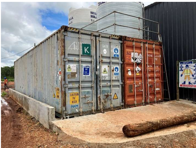
Plate 3-1: CCA store at pole plant (note minimal front side bunding or cover from elements)
