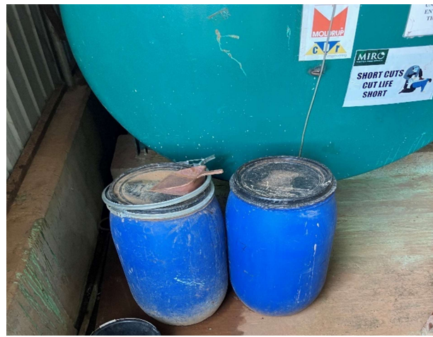
Plate 3-2: Stockpiled CCA waste residue at pole plant
